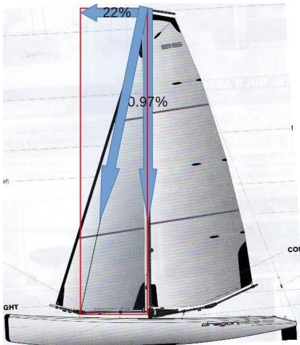
Mast #1 is tuned with compression and moderate forward tension. The forward tension is 22% of the trim load and the compression is 97%. Given the forestay masthead attachment point is ahead of the mast, tuning only the forestay (backstay slack) should *bow* the mast *aft* with the center of the bow somewhat above its mid-point because of the stepping arrangement.
