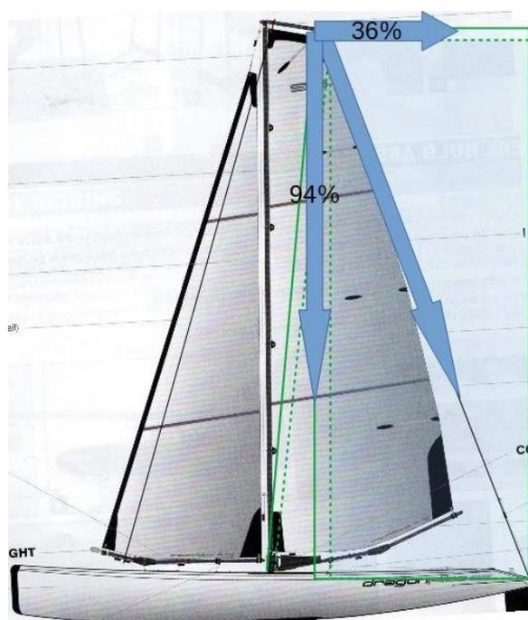
Because of the crane, Mast #2 is tuned in compression and torsion. Rather than *bowing*, it acts as a pinned, tip-loaded cantilever and *bends* from the deck to the tip.
