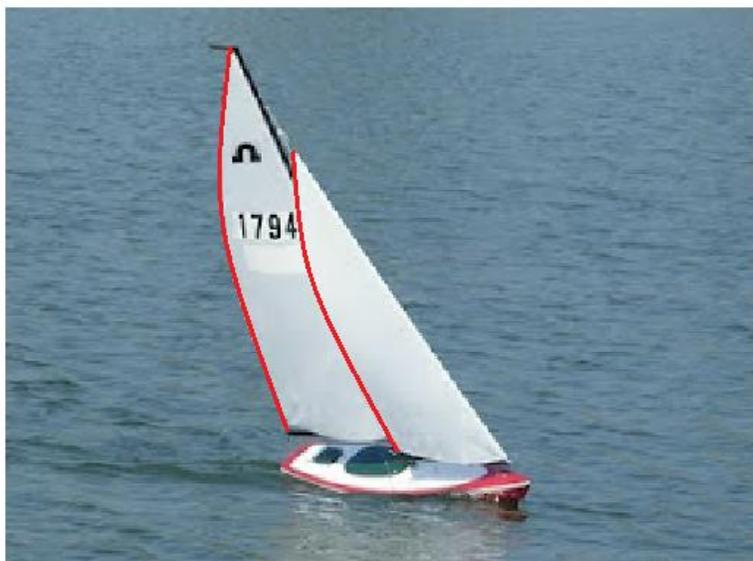
A pretty-well tuned Soling. Note the curves of the mainsail leech and the jib leech- they closely match. The mainsail boom is pointed *juuuust* inside the aft deck corner, and the jib boom juuuust inside the shroud. Note the sails have a fair amount of twist- the leeches are “open” for power.
