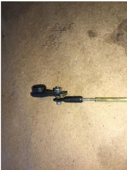
Note the rudder post has a flat section to grab the set screw on the steering arm. It will provide more grab for the steering arm and prevent the rudder from slipping out of the boat if the set screw starts to loosen. You will get a little warning before you lose the rudder.
